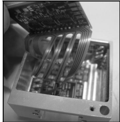
FIGURE 10 – FLEX CIRCUIT INSTALLED
