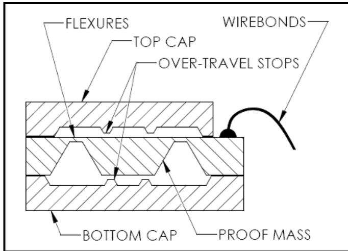
**FIGURE 3 – SENSOR CROSS-SECTION**
