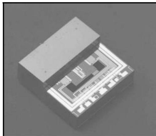
**FIGURE 2 – PR SENSOR ELEMENT, UNCOVERED**
