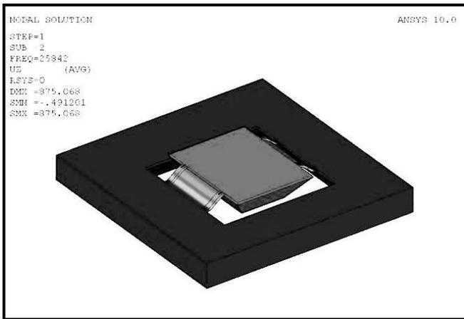
FIGURE 7 – FEA MODEL OF SENSOR ELEMENT
