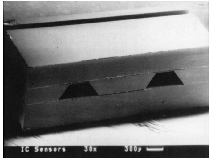
**FIGURE 5 SECTIONED SENSOR ELEMENT**
