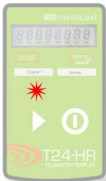
The handheld has the ability to configure an acquisition module to match the handhelds own radio channel and encryption key settings.
