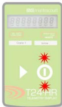
The handheld has the ability to perform a system zero on a remote acquisition module. This may be useful after installing new modules and enables system zero to be set without the need for a PC/laptop and T24 Toolkit.
