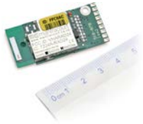
T24-TA Wireless acquisition for temperature measurement equipment
