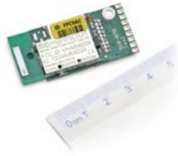
T24-PA Pulse to wireless telemetry converter
