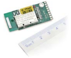
T24-IAe Current to radio telemetry converter
