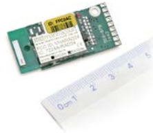
T24-VAe Voltage to wireless converter
