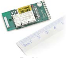
T24-RAe Wireless potentiometer for displacement sensor.
