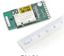
T24-PAe Pulse to wireless telemetry converter
