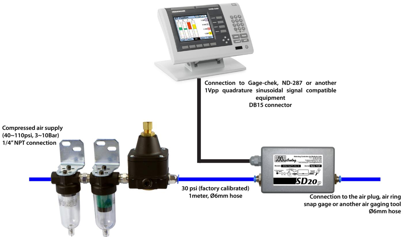
Connect the filters and air regulator assembly to the compressed air network (40~110psi, 3~10Bar) and the SD20-p1Vpp / TTL conditioner. The air supply should be free of lubrication and have low humidity and impurities. Clear the particulate filter (5 µm) and the coalescing filter (0.05 µm) whenever necessary. The instrumentation pressure regulator output is factory set and should **NOT** be changed by the user.
