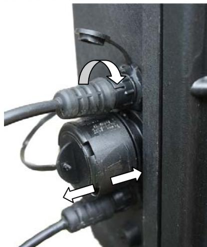
The PP1 110 - 240Volt AC input has a sealing cap for when it is not connected to the mains. The sealing cap is removed by pushing the outer sleeve towards the case and pulling the cap out.
