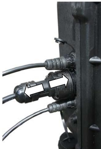
To insert the mains cable input simply align the two parts using the locating grooves on the connector and push in until the outer sleeve locks; to remove again repeat the same procedure as to remove the sealing cap.
