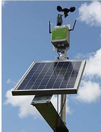
*A high capacity battery pack with solar and mains charging providing long term 12 Volt power for field applications, specifically Remote Data Collection (T24-RDC)*
