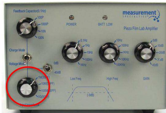
**Input Attenuator Switch (voltage mode)**
