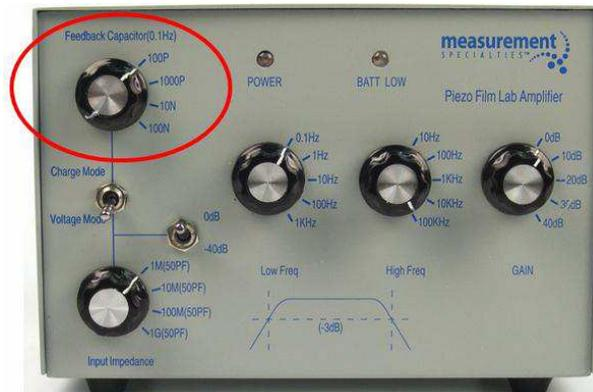
**Input Impedance Selector** (voltage mode)
