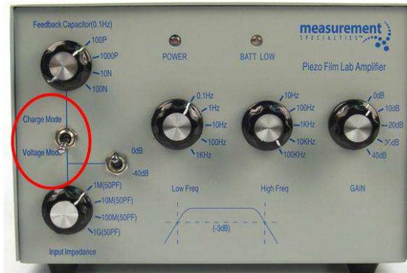
**Feedback Capacitance Selector** (charge mode)
