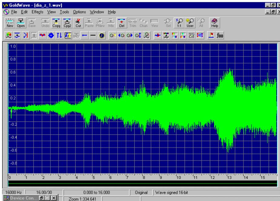
Figure 4: Microphone output, 200 to 1000 Hz sweep, with screws rattling on diaphragm
