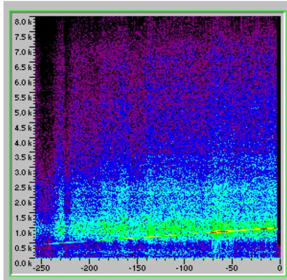
**Figure 5: Spectrogram from trace of Fig 4, showing relatively uniform noise generation over 500 to 1000 Hz approx**
