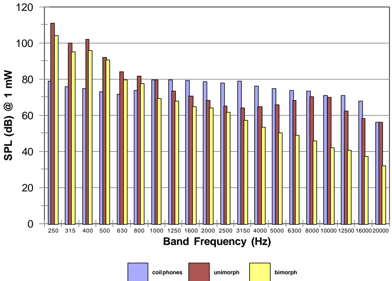
in level around 10 kHz compared with the bimorph (which subjectively made the unimorph sound louder and "brighter" than the bimorph version).
