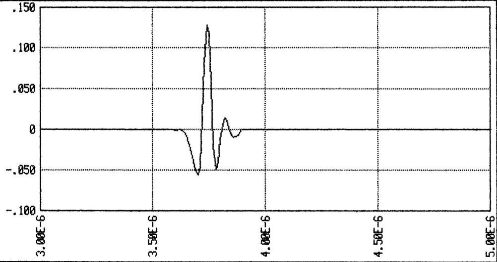
DRIVE SIGNAL TO 52um PVDF VIA X100 PROBE
