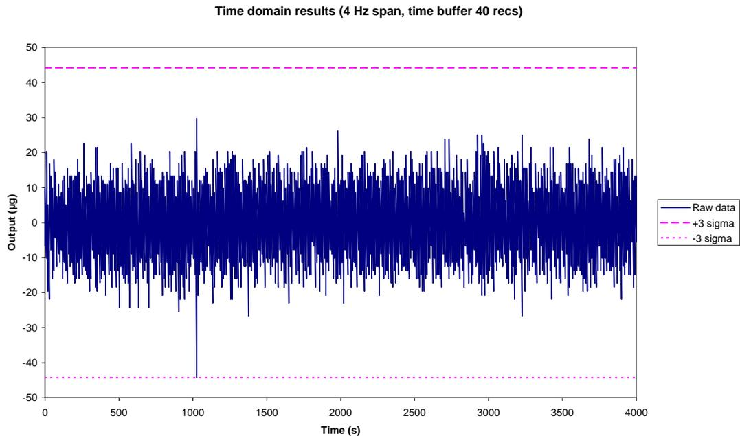
From the above waveform, it is clear that although signals in the  $1 \mu\text{g}$  magnitude range may be resolvable in the frequency domain, it would be virtually impossible to detect these from simple inspection in the time domain. (Note as an example: it would be very difficult to conclude whether the negative-going transient signal at 1025 s in the above trace, value  $-44 \mu\text{g}$ , resulted from pure electronic noise, or was a valid acceleration event).
