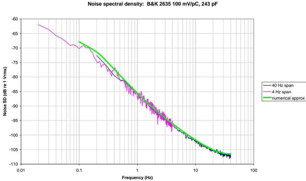
As might be expected, the noise increases in magnitude as the frequency decreases. It appears to "level out" at the upper end. Note that the typical sensitivity of the Minisense component begins to increase at higher frequencies (due to resonance at 75 Hz), and has already reached +3 dB at approximately 42 Hz.
