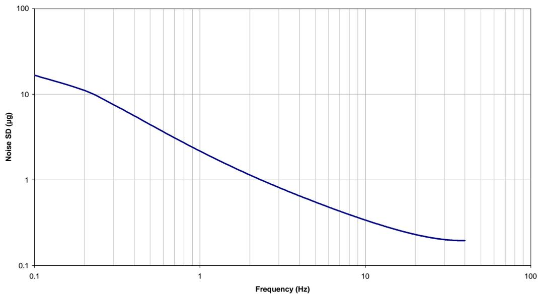
Note that the effective noise floor is quite impressive: around  $2 \mu\text{g}$  at 1 Hz, and around  $0.3 \mu\text{g}$  at 10 Hz. However, in any real application, the full time-domain picture may be as or more important than the above spectral plots.
