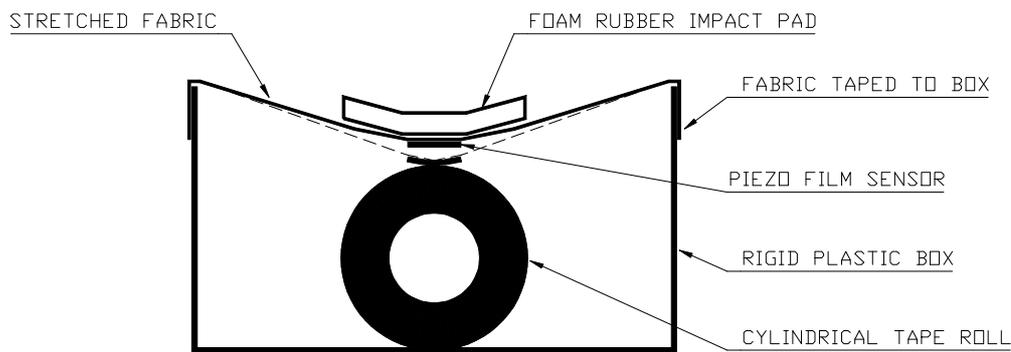
IMPACT SENSOR TEST ARRANGEMENT
