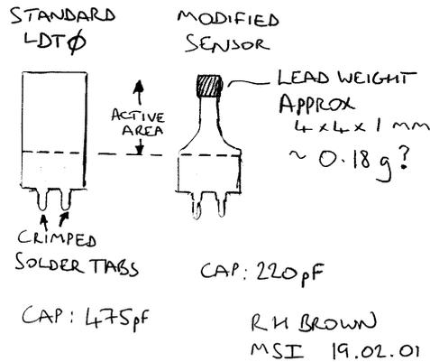
Although the device was not calibrated, various shaking actions were performed using the sensor connected to a 100 M resistive load, giving low frequency -3 dB roll-off at 7.5 Hz. A higher value would be preferred, but a 100 M x100 'scope probe was quick and easy way to test the device. 220 M or 470 M would be more suitable values.
