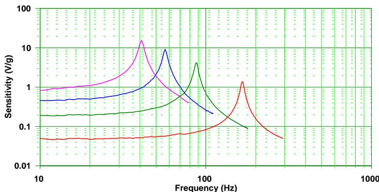
It can be seen that a sensitivity in the region of 0.5 V/g can be reached at baseline, when a resonance peak at around 58 Hz is achieved by adding mass to the tip.
