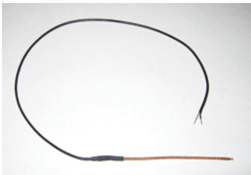
Fig. 2. A piezo cable in which the sensitive element (the portion sheathed in braided copper) is designed to react to lateral compression.
