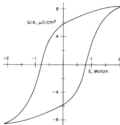
Figure 4.12 Typical hysteresis loop between electric displacement ( $Q/A$ ) and electric field ( $E$ ) for ferroelectric polymer.
