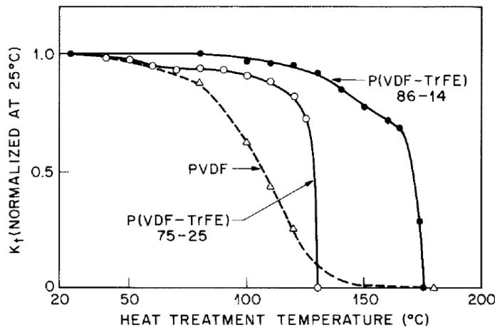
**Figure 11.9** Thermal stability of piezoelectric activity in PVDF and P(VDF-TrFE); the value of the coupling factor  $k_t$  measured at room temperature after annealing is plotted as a function of annealing temperature. Annealing was carried out for 10 min at every temperature. Redrawn and adapted from H. Ohigashi, *Japan J. Appl. Phys.* **24 Suppl.** 24-2 (1985) 23.
