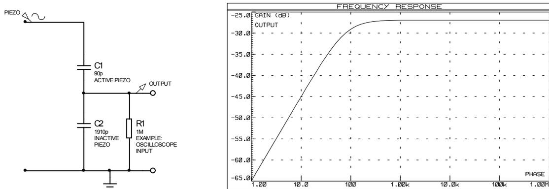
The cut-off frequency remains unchanged at 79 Hz (because the total circuit capacitance is the same), but the "gain" has reduced to  $-27$  dB in the flat region of the curve. In other words, the true voltage developed by the active segment in isolation from any load is reduced by a factor of 22 (which is the same as the ratio of active to total length).
