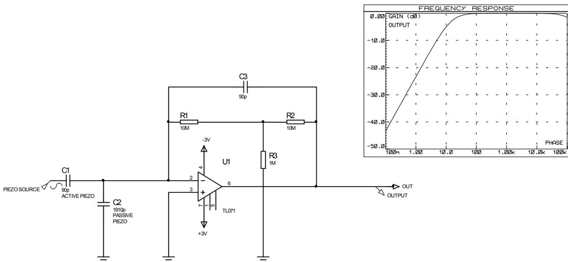
To illustrate the insensitivity of the circuit to capacitive load on the input, the simulation is run again below, changing the value of C2 from 1910 pF (as used in above examples) to 100 nF (equivalent to around 111 m of cable). Note the effect on higher frequencies.
