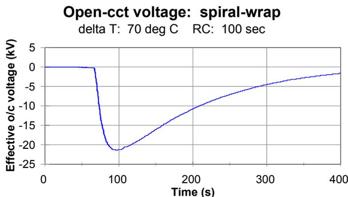
All three cables demonstrate very high open-circuit voltage sensitivity to thermal transients, although the long thermal time constant would prevent such sensitivity being observed in normal circuits with much shorter electrical time constant. Differing jacket material and thicknesses, and different mounting configurations, will significantly affect the actual thermal time constant observed in a given detection situation.
