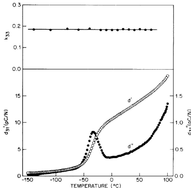
**Figure 5.27** Plots of complex piezoelectric constant  $d_{31}^*$  and electromechanical coupling factor  $k_{33}$  of PVDF as a function of temperature.
