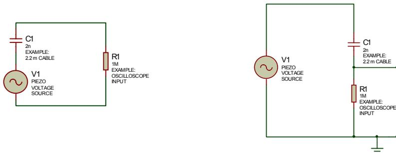
An active model can be produced, where the voltage source V1 in the diagrams above is replaced by a sine generator, and a frequency response curve generated by comparing the output observed across the 1 M resistor with the input:
