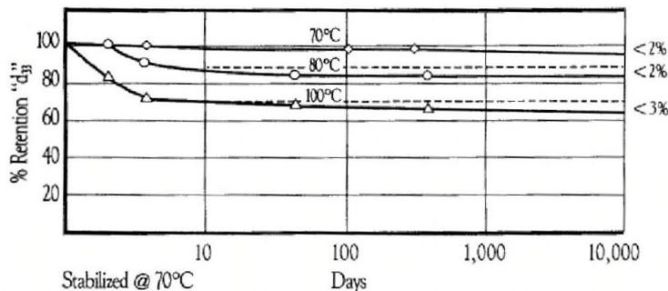
It should be noted that the storage temperature required to bring about a complete depolarisation of piezoelectric PVDF has been estimated as 200 °C, which is above the melt temperature for the crystalline beta-phase (180 °C).
