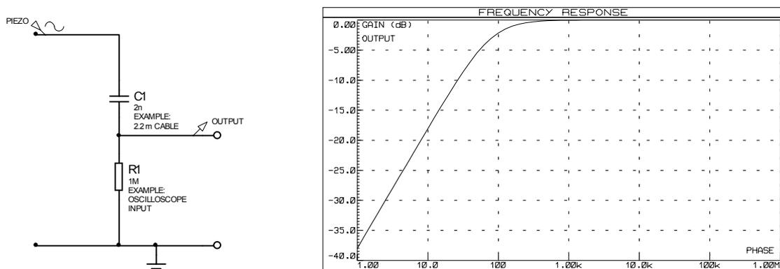
In this case, for a 2.2 m long section of cable with capacitance 2.0 nF, the cut-off frequency (to -3 dB, or to 0.71 of peak value) lies at 79 Hz.
