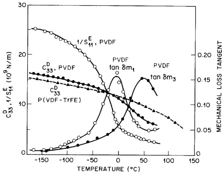
**Figure 11.7** Temperature dependence of mechanical properties of PVDF and P(VDF-TrFE) (VDF/TrFE = 75/25). Redrawn and adapted from *J. Appl. Phys.* 47 (1976) 949.
