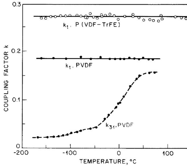
**Figure 11.8** Temperature dependence of electromechanical coupling factors  $k_t$  and  $k_{31}$  for PVDF and P(VDF-TrFE) (75/25) [14, 28].
