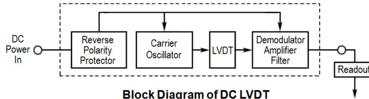
The carrier oscillator produces a constant amplitude sine wave to excite the primary of the LVDT. The sinusoidal excitation provides superior performance to square waves.
