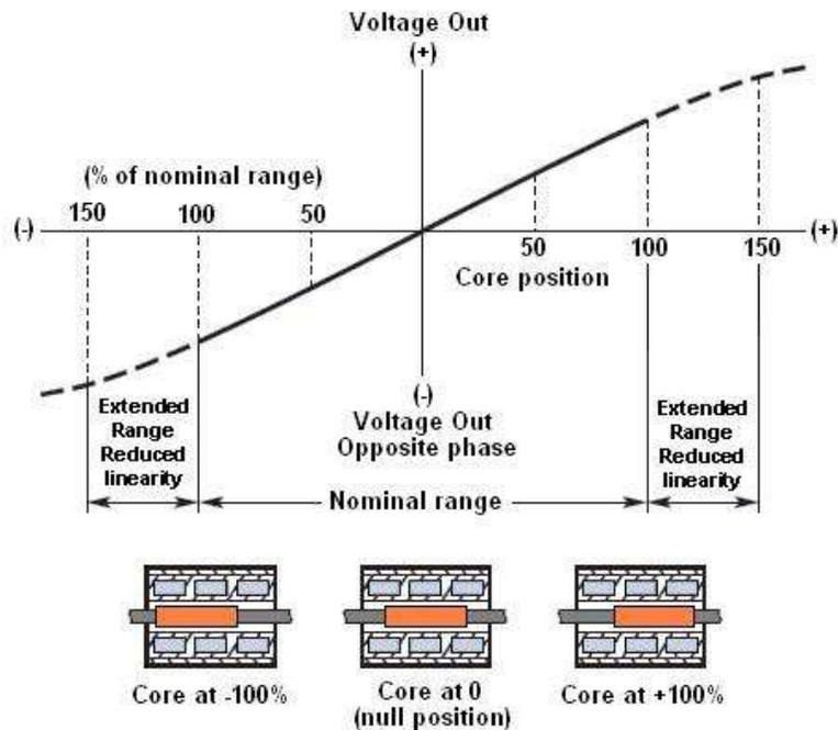
**TE CONNECTIVITY LVDT DESIGN AND CONSTRUCTION**
