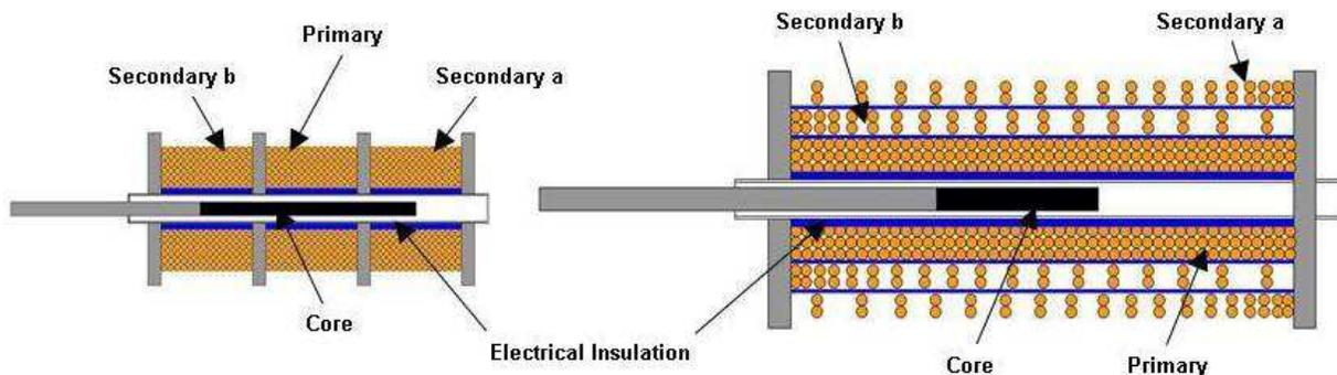
LVDT cross-section. short stroke ( $\leq 0.2$  inch)
