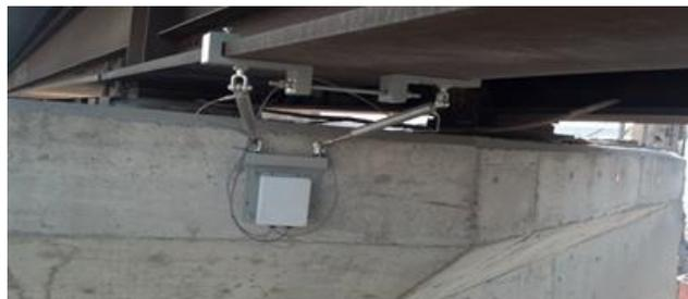
As can be seen in the photo above showing a pier-to-bridge interface measurement application, the LV-45s are hard fixed to the pier and to the bridge, using ball joint swivel rod ends to take up any misalignment during initial installation. The system can measure position changes in all three axes and can track those changes over time to show short and long term trends and highlight potential problems or incipient failures before they take place.
