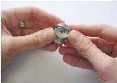
2. Remove the cable gland nuts and plastic inserts from the bodies of the EMC glands and slide them onto the ends of the cables.
