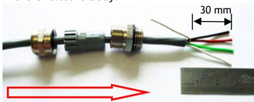
4. Strip 2mm of insulation from the individual wires before tinning the ends and soldering to the PCB.
