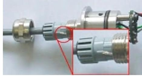
7. Push the plastic insert fully home and check to ensure that no strands from the drain wire are visible; slide the gland nut into place and tighten so that the cable is firmly gripped by the lining of the plastic insert.
