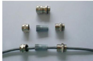
3. Lay the cable drain wire back along the cable outer insulation and pass the prepared end of the cable through the gland shell on the enclosure body.
