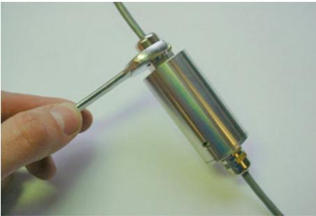
8. Taking care not to damage the EMC 'O' ring, and making sure that the cable drain wire passes back through the gland, carefully assemble the enclosure body with the PCB mounted on it, to the enclosure cover and fit the two retaining grub-screws.
