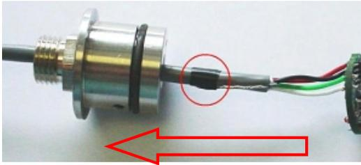
6. Slide the EMC gland plastic insert into place ensuring that the drain wire passes between the plastic insert and the gland shell and ends at the step in the insert; note that there are slots in the shell to accommodate the raised areas on the outside of the plastic insert.
