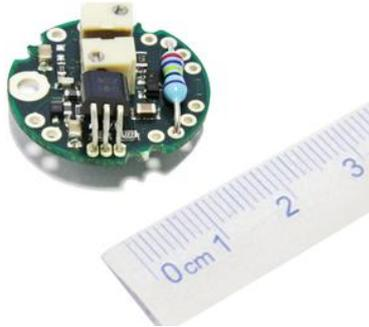
*A range of high performance robust signal conditioners in a miniature OEM format and designed specifically for fitting inside load cells*
