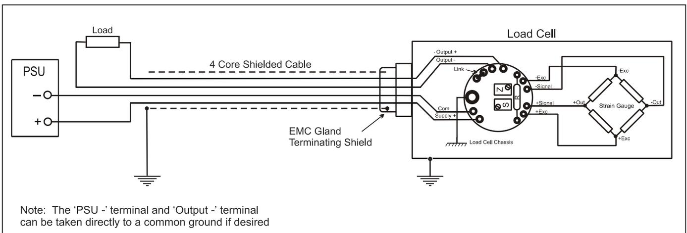
Take note of the grounding arrangement particularly the bolt hole which capacitively couples the common of the ICA electronics to the strain elements in the load cell which improves the EMC performance.
