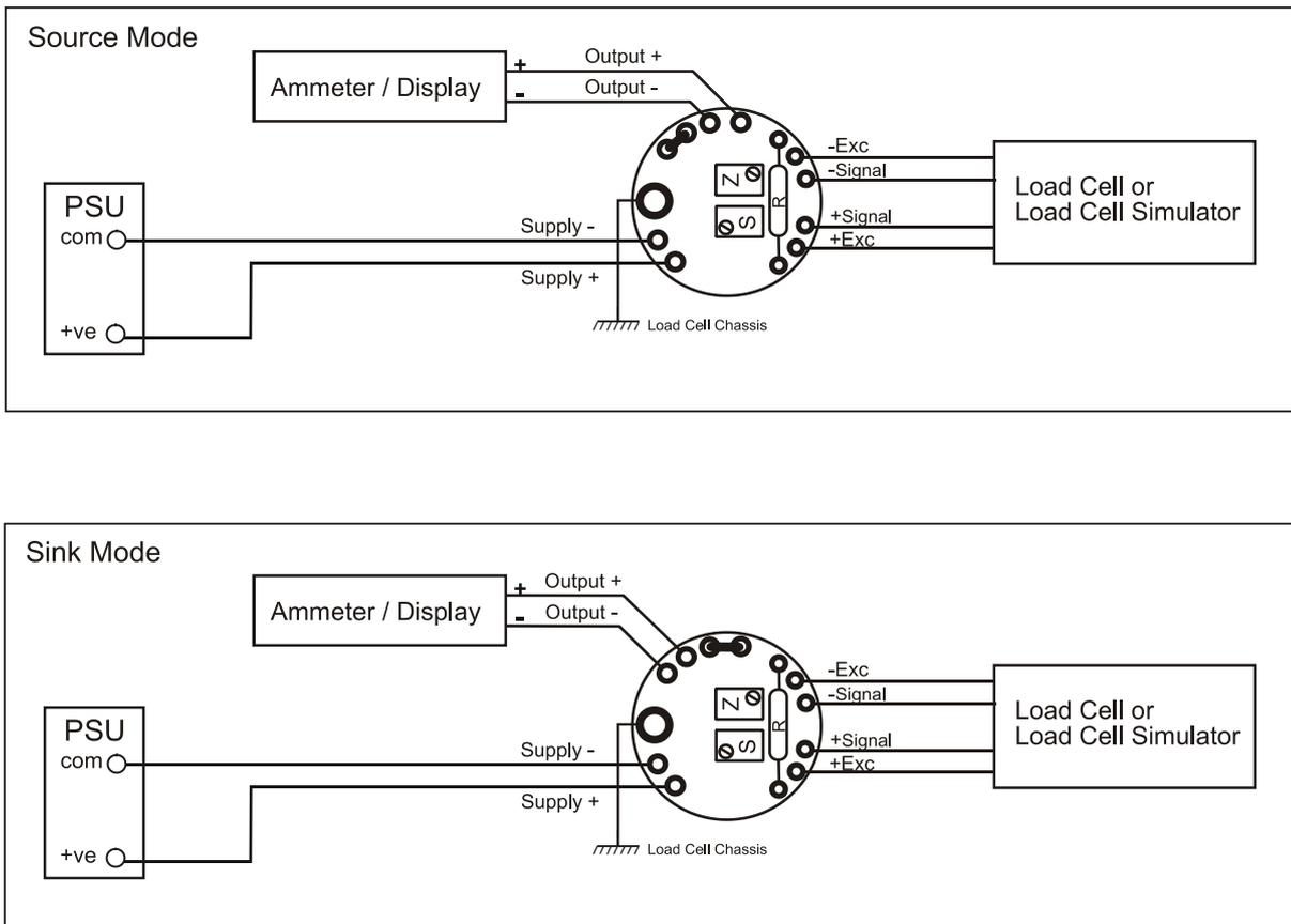
1. Apply the known **low** calibration conditions (weight, force or mV/V). This may be zero if required, and set the output to 4mA using the 'Z' potentiometer. Note the exact reading.
