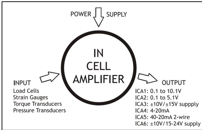
The ICA is a Strain Gauge Amplifier, converting a strain gauge input to a Volt or mA output - otherwise known as a Signal Conditioner.
