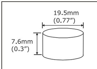
The module is designed to fit in the strain gauge pocket. Use the 2.1mm hole to secure the unit if required. The mounting hole will accept an M2 screw or American equivalent #0-80. Important Note: DO NOT USE #2 screw size.
