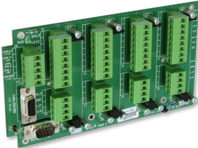
*Designed to enable the easy connection of up to 4 load cells and 4 DSC cards to a multi-dropped digital communications bus*
