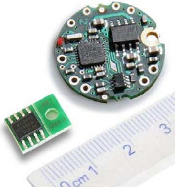
*Miniature format designed specifically to be incorporated directly into strain gauge sensors such as load cells, pressure transducers and torque sensors*
