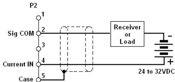
4-20mA OUTPUT USING AN EXTERNAL LOOP SUPPLY
