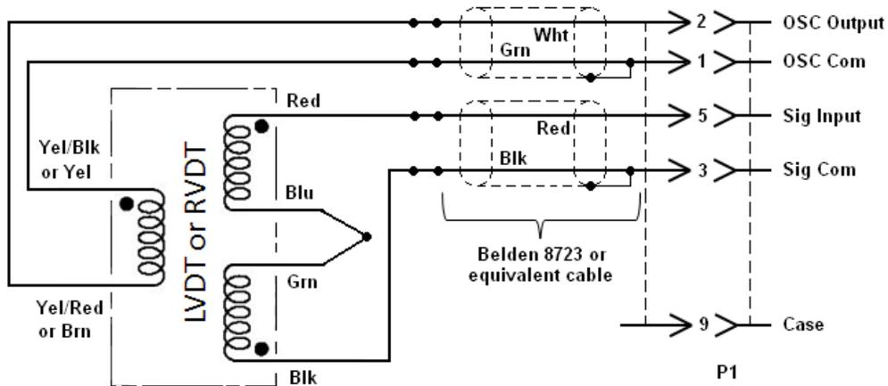
TRANSDUCER WITH LEADS AND SPLICED CABLE
