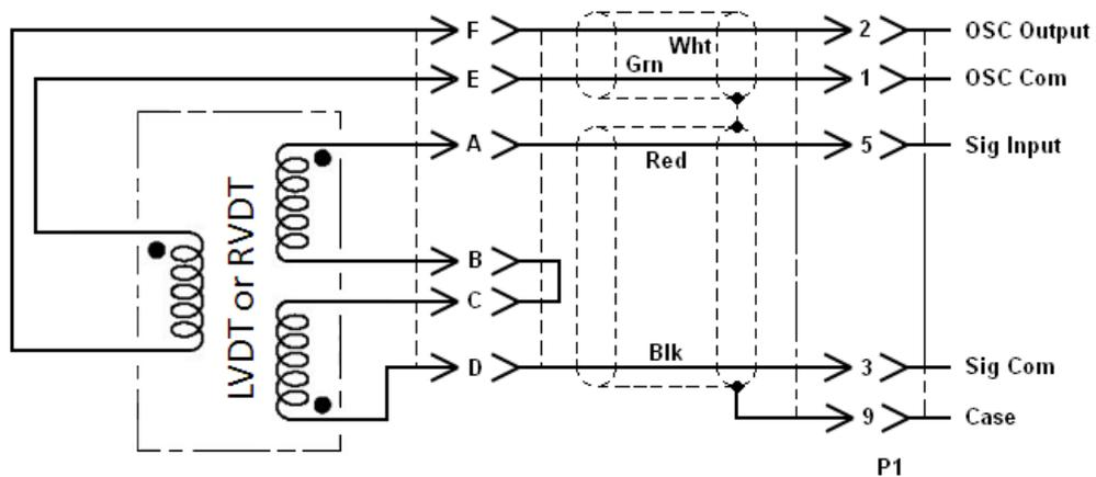
TRANSDUCER WITH CONNECTOR AND JUMPER CABLE
