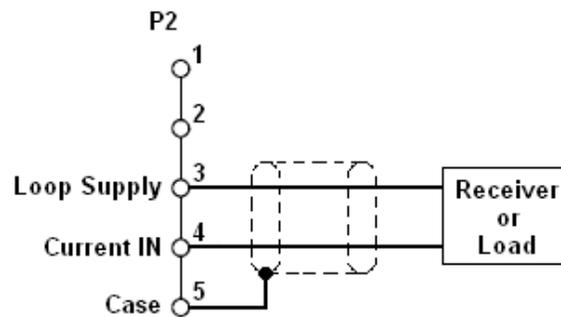
4-20mA OUTPUT USING THE INTERNAL LOOP SUPPLY
