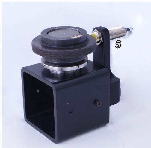
Picture 1-2. Detail of the measuring plug and the inductive sensor IS101
