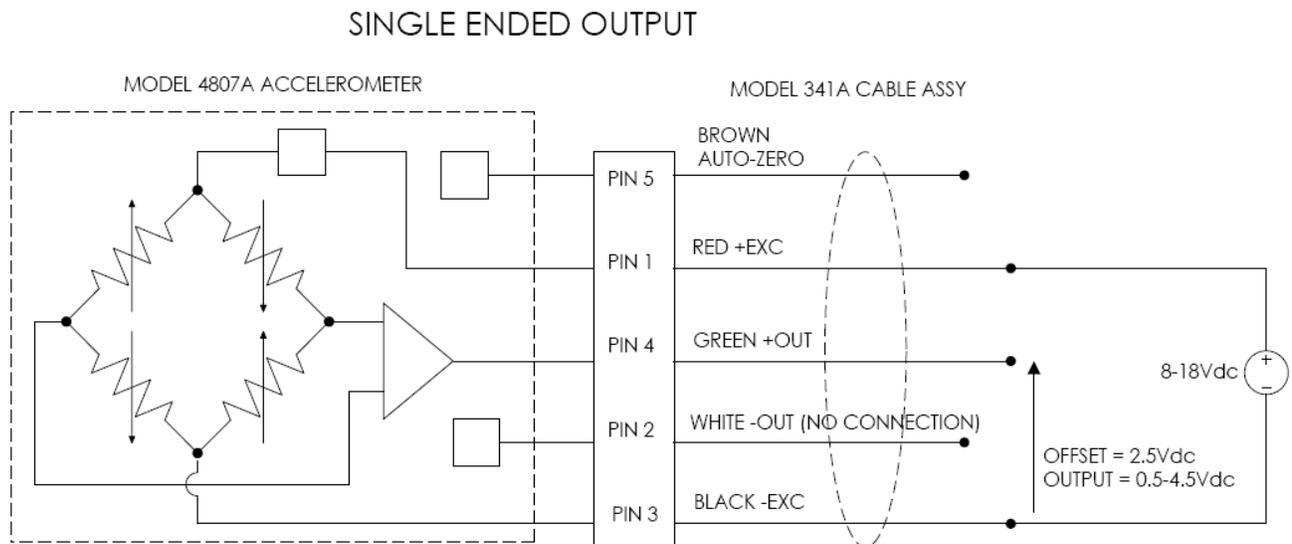
Model 340A cable can also be used if auto-zero function is not required.
