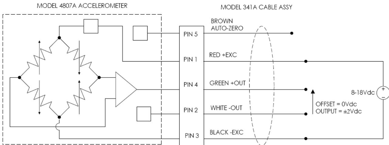
Model 340A cable can also be used if auto-zero function is not required.
