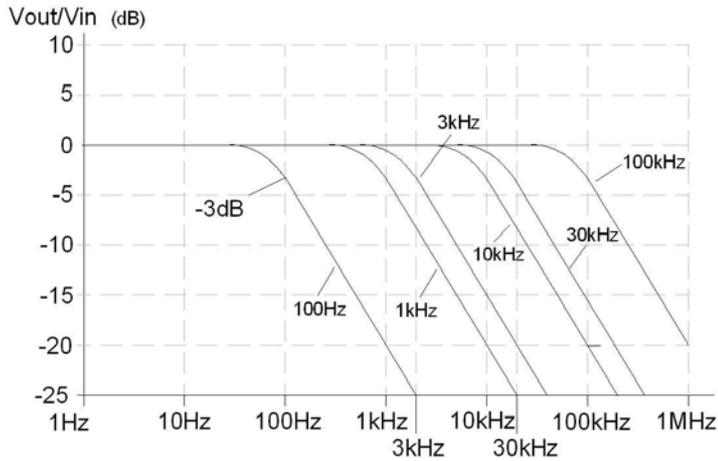
Figure 3-5. Attenuation Curve of the Low-pass Filter
