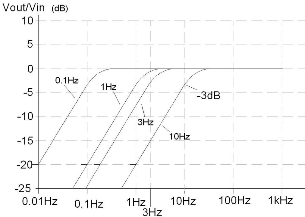
Figure 3-4. Attenuation Curve of the High-pass Filter
