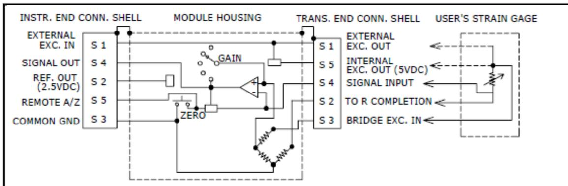
Figure 12: 142 Quarter-Bridge Strain Gage Wiring Diagram
