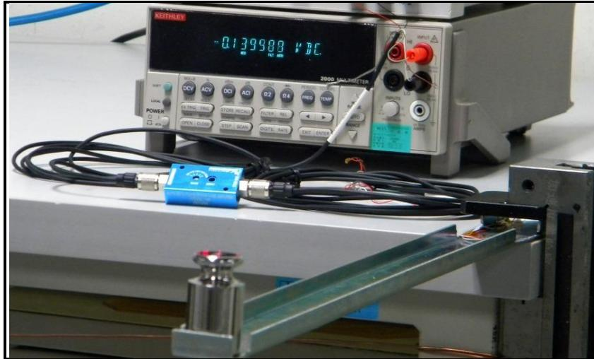
Figure 13: Strain Gage Measurement on Cantilevered Bar
