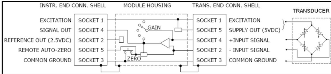
Figure 2: 140 Wiring Diagram
