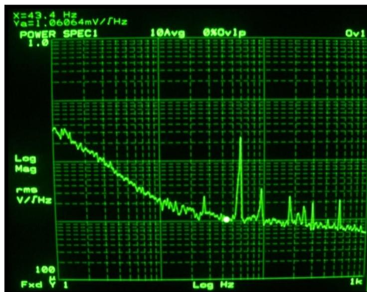
Figure 3: PSD of 3022-010 PR Accelerometer Plugged into a 140
