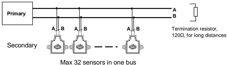
**If communication fails to work, switch A and B polarity at Primary end.**
